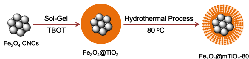
Scheme 1. Schematic Illustration of the Synthetic Procedures for the Preparation of Modified \text{Fe}_3\text{O}_4@\text{mTiO}_2\text{-80}
